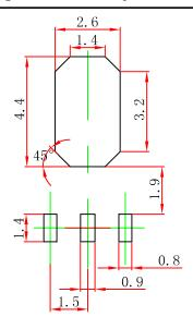
Note: 1.Controlling dimemsion写in写milimeters. 2.General tolerance: ±0.05mm.
